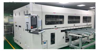
Automatic Lamination and Welding Machine: Welds cell strings using bus bars.
