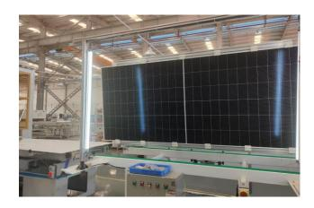
**IV Tester**: Tests the power and electrical performance of components.
