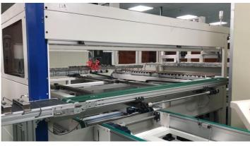
Layout Machine: Arranges and stringwelds battery cells on photovoltaic glass.
