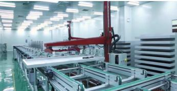
**Curing Line**: Cures the silicone by maintaining constant temperature and humidity.
