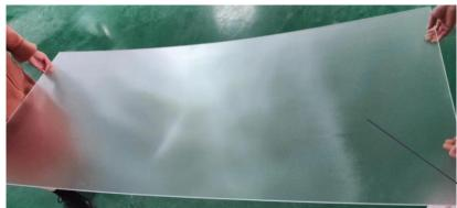
Check the impact strength of the glass. Free fall from a height of 1 meter for three times without damage
