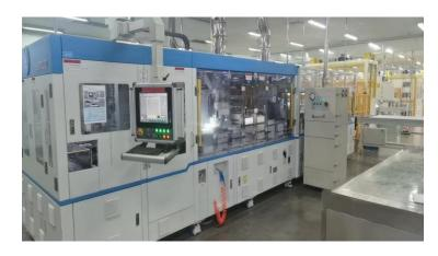
**String Welder**: Welds and connects battery cells in series to form cell
