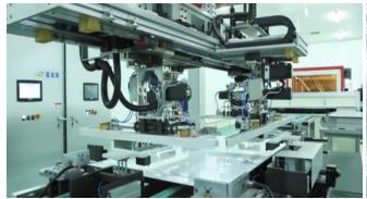
**Gluing and Framing**: Applies glue and assembles the frame.
