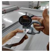
Weight measurement and wall thickness inspection of the frame
