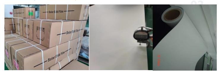
Inspect the gram weight, thickness of EVA and backsheet, and check for no mechanical damage.
