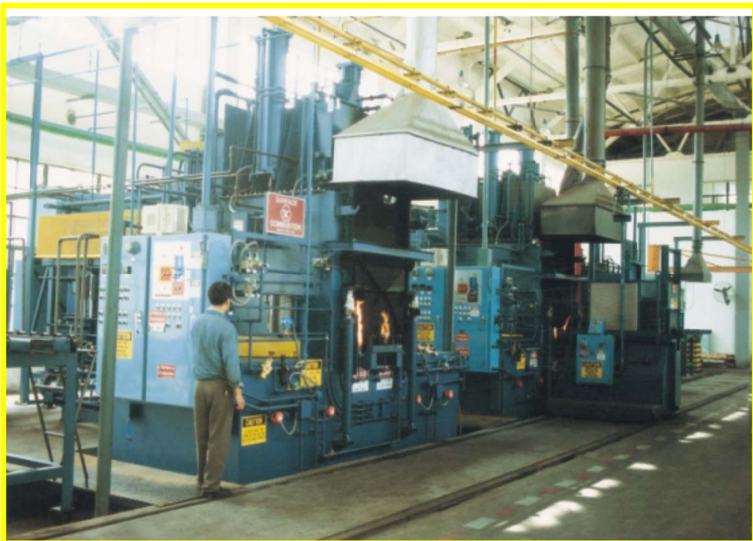
Heat-treatment Furnace with Nitrogen Base Controllable Atmosphere
