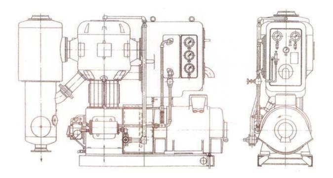
Length: approx. 2800 - 3015 mm (Depending on type of motor) Height: approx. 1975 mm Width: approx. 1000 mm
