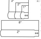
\*Z: 8" paddle must be shortened according to the pipe diameter. The installed paddle must not touch the pipe walls.
