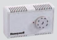
The H6045A1002 single-stage duct hygrostat and the H6120A1000 single-stage room hygrostat are designed for monitoring relative humidity in air conditioning systems and climatic chambers and for controlling air humidifiers and dehumidifiers in indoor swimming pool buildings. Both devices have a dust protected microswitch with a high switching capacity. Thanks to their simple and robust construction, they offer a low-cost solution for heating, ventilation and air-conditioning systems.
