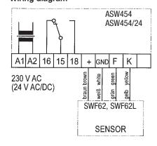
In case of malfunction, a sensor error can be ruled out by checking the resistances between the connecting wires of the sensor. Sensor SWF62 or SWF62L must be disconnected and checked with a suitable ohmmeter between the individual connecting wires:
