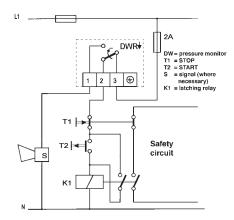
Where the above lock circuit is used, the requirements of DIN 57 116/VDE 0116 are met if the electrical equipment (such as contactors or relays) of the external interlock circuit satisfy VDE 0660 or VDE 0435.
