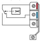
At falling flow switching from red - white to red - blue at rising flow switching from red - blue to red - white.
