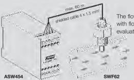
The flow in fluids can be monitored reliably with flow sensors SWF62 and SWF62L and evaluation unit ASW454.
